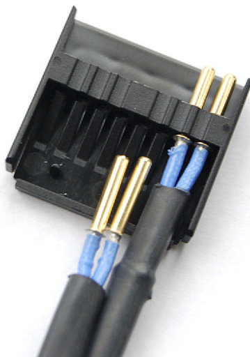
Figure 48: Inserting additional probe wires
